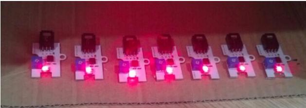
5. Lead the photosensitive modules to the outside of the box via DuPont lines, connect them in parallel via the soldering iron and fix them via the sol gun.
